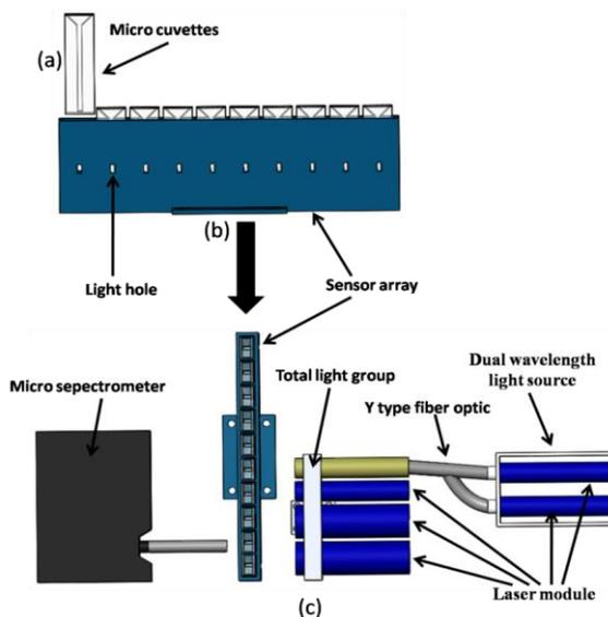
Fig. 1: Illustration of the optic cross-responsive sensor array device. (a) The structure of the micro cuvettes; (b) The structure of the sensor array that consists of 10 chemically responsive spots which are injected in micro cuvette when detecting; (c)The schematic diagram of the device.
